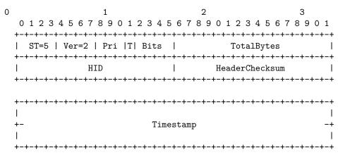
As ST would be incompatible with IP, the next version number was assigned to identify its packets. Ever since then, the number 5 was reserved for ST in the IP version field (layer 3) and protocol number (layer 4) field. The idea is that routers could differentiate packets or that IPv4 packets could carry encapsulated ST packets, where the number 5 would show up as an upper layer protocol. Since RFC762 we can see number 5 assigned in "protocol numbers":
